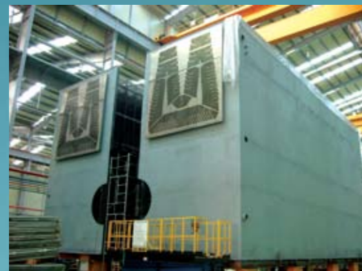
Surface Condenser under Assembly
